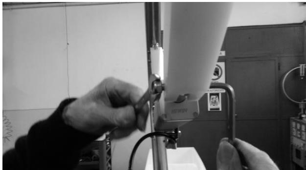
Now connect the loop junction blade. Spread the anti-oxide paste (provided) inside the joint before installing the retaining bolts.
