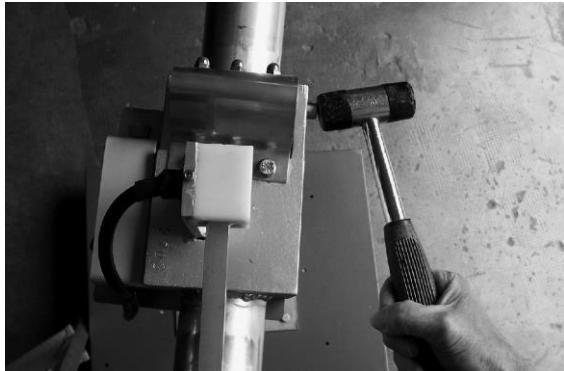
When the pin is fully engaged, install the washer and the bolts. then tighten them. A 6mm (0.23in) wrench is provided for this.
