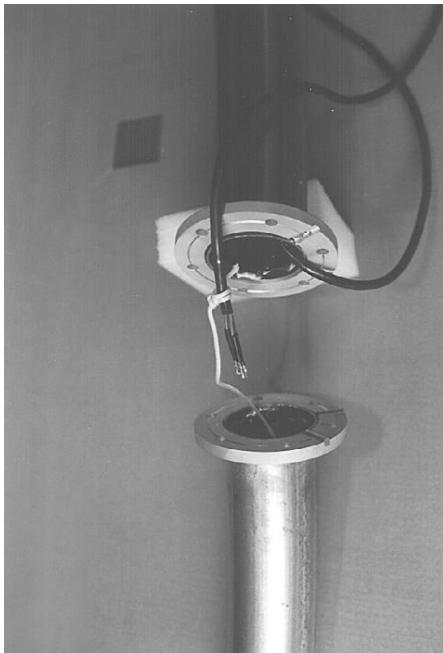
The same operation is required to assemble the other semi-loop. Before joining the second semi-loop, it's necessary to feed the actuator power line through the two aluminum tubes and flanges. This can be done by hooking the power line to the string already inside the tube.
