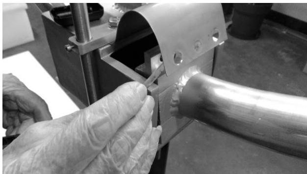
Fit the washer and the bolts. Tighten them with a wrench.
