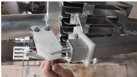
After the piston-head is in place, install the fix cap head hexagon socket drive screw with self-locking nut. Tighten the nut until it reaches the surface of the isolated arm. **Do not force it.**
