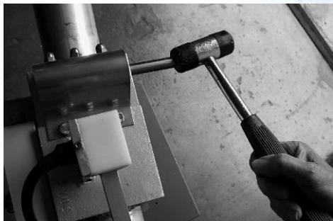
Using a plastic hammer, fully insert the pin. Do not use excessive force. If necessary, gently move the semi-loop until the pin is in place.
