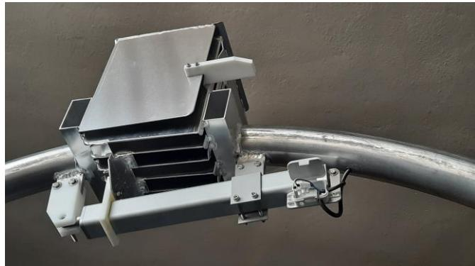
Now connect the semi-loop junction blade. Spread the anti-oxidant paste before installing the retaining bolts.
